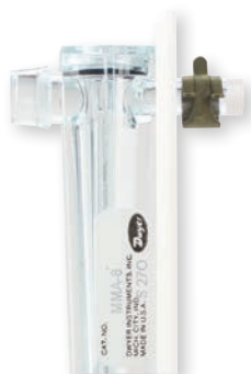
Spring retainers on connection tubes secure panel mounted MMA. Compression union, P/N A-327 shown.
