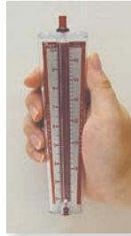
Hold this way for low scale reading
